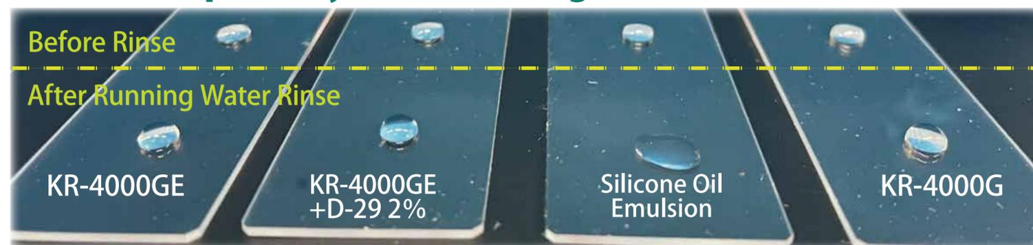
\* The upper side is unwashed, and the lower side is after 10 minutes of running water rinse, wiping with tissue, and then dripping 0.02 mL of water onto it.
