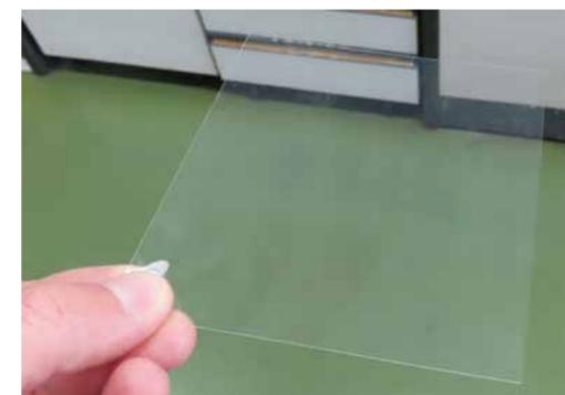
A composition containing 2 wt% of a photoinitiator is applied to a PET film and cured at 600 mJ/cm<sup>2</sup> under N<sub>2</sub> atmosphere.
