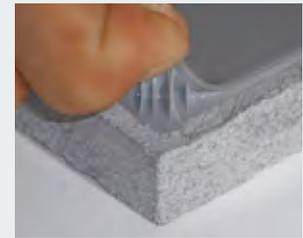
Following application, lift one edge slightly to confirm the string like appearance of the adhesive layer and no less adhesion.
