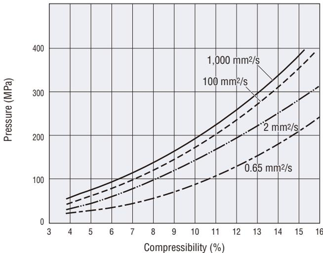
Fig. 15-2 Pressure and compressibility of DM-FLUID (25°C)
