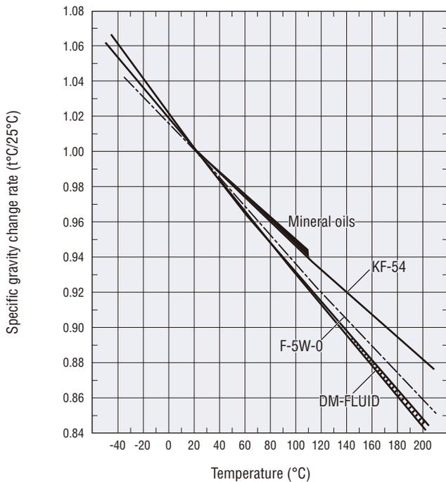
**Fig. 10 Correlation between temperature and volume ratio**
