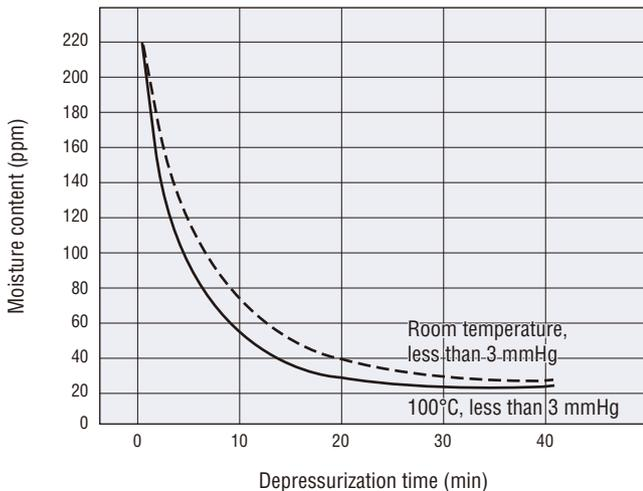
Dehydration conditions: A sample of silicone fluid (fluid depth: 10 mm) was put in a glass container (50 mmf). It was then depressurized to less than 3 mmHg and a continuous dehydration process was used, once at room temperature and again at 100°C.
