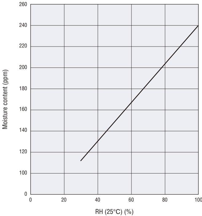
**Fig. 30** Moisture absorption speed of DM-FLUID-50cs
