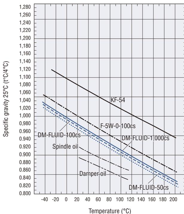
**Table 6 Specific gravity change rate by temperature (t°C/25°C)**
