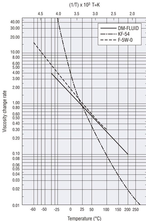
**Fig. 4-2 Viscosity change rate by temperature (0°C to 50°C)**
