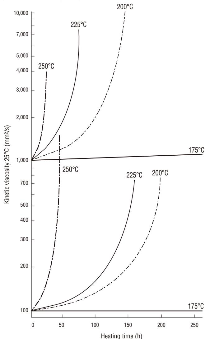
**Fig. 13 Heating loss of DM-FLUID-100cs**
