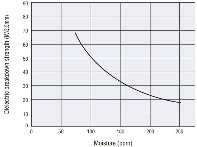
Fig. 21 DM-FLUID-50cs: moisture content and dielectric constant
