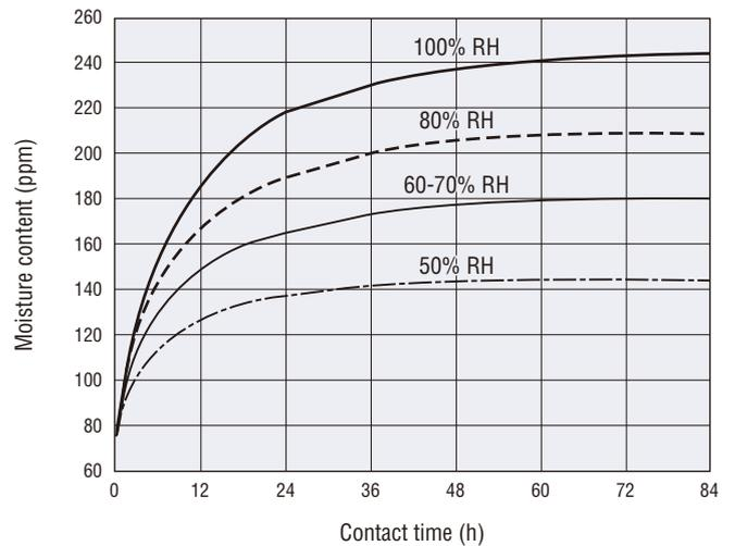
Measurement conditions: Roughly 300 g of DM-FLUID-50cs was collected in a 1 liter beaker. A glycerin and water solution was used to measure the differences in the amount of moisture absorbed in atmospheres of varying relative humidity values. Moisture was measured by the Karl Fischer method.
