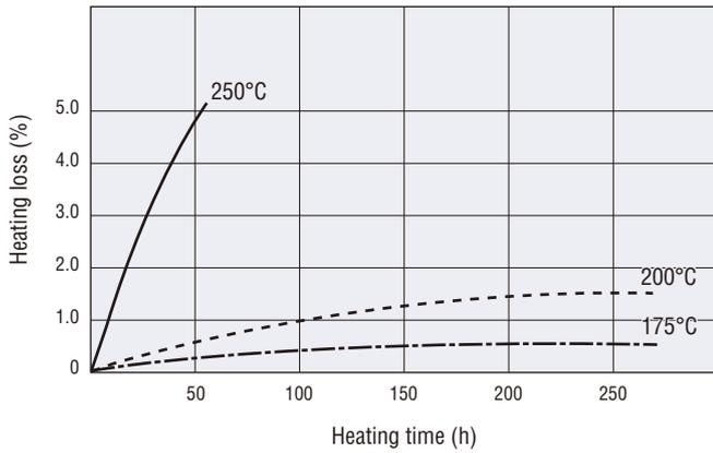
**Fig. 14 Heating loss of DM-FLUID-1,000cs**
