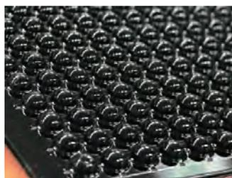
Photo: Microlens by transfer molding
