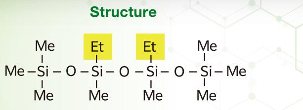
Silicone fluid in which a portion of methyl group is replaced with an ethyl group
