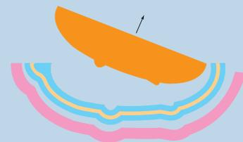
Once the replica resin has been completely cured, remove it from the mold and the replica is finished.
