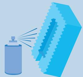
Spray the silicone rubber mold with a releasing agent as necessary.
