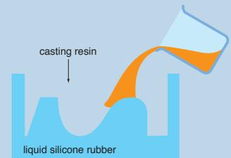
Pour the casting resin into the silicone rubber mold and let it cure. You can lengthen the life of the silicone rubber mold if you apply a releasing agent as necessary.
