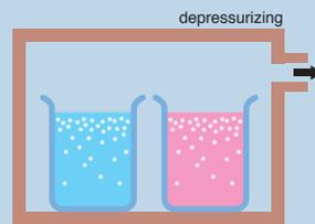
Depressurize and defoam the specified amount of casting resin.
