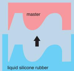
Once the rubber cures completely, pull the master from the frame. The silicone mold is now complete
