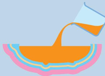
Once the backing material has completely cured, remove the master. Pour a casting resin into the silicone rubber mold and allow it to cure.
