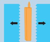
Split the cured mold, and remove the poured item. Cut off the gate and file down the area.
