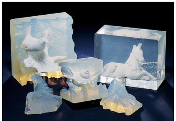
Transparent and translucent liquid silicone rubber moldmaking
