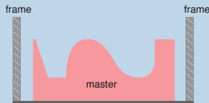
Place the master within a frame and secure it to the bottom.
