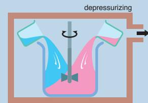
Mix the defoamed casting resin.
