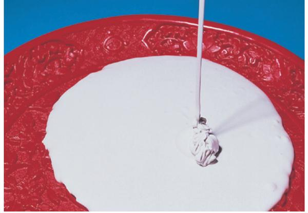
Liquid silicone rubber flows easily into the tiniest of recesses.
