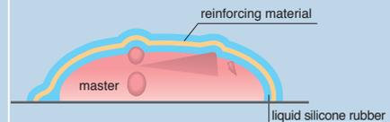
Once the liquid silicone rubber has hardened but is still slightly sticky, apply reinforcing material such as glass cloth or gauze, and then apply an additional two to three coats of liquid silicone rubber.
