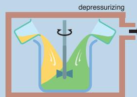
Thoroughly mix the base compound with a curing agent while depressurizing and de-airing.
