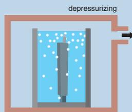
Depressurize and defoam, and then allow the mold to stand for the specified time. If you are using an addition-cure material, then the curing time can be shortened by applying heat.
