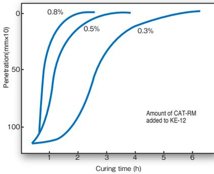
Figure 2 Amount of curing agent added and curing speed with KE-1417 (condensation-cure type) at 23°C.
