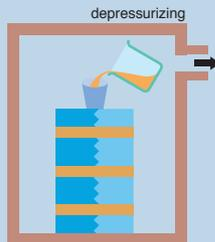
Pour in the casting resin which has been mixed via the plastic stopper under a depressurized state.
