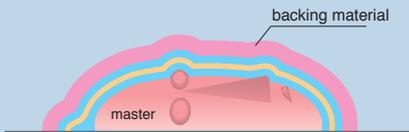
Once the liquid silicone rubber has completely hardened, apply a backing material such as gypsum or polyester to enhance the strength of the mold.
