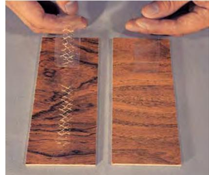
Separation test with cellophane tape on plywood
