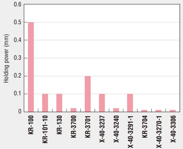
Backing: polyimide film, 25 μm thick; PSA thickness: 30 μm, 40 μm (KR-100, KR-101-10, KR-130).
