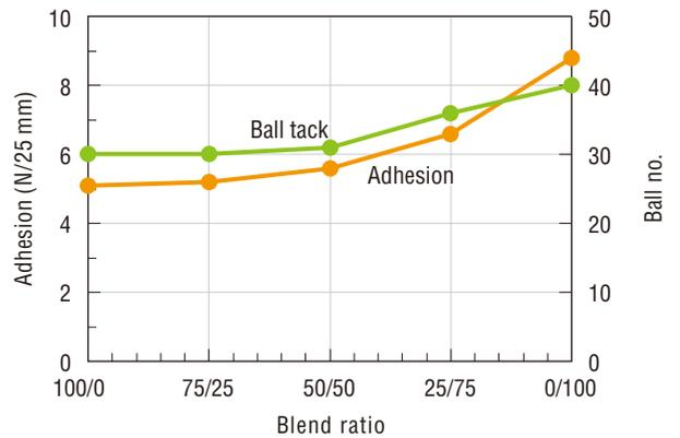
Backing: polyimide film, 25 μm thick; PSA thickness 30 μm.
