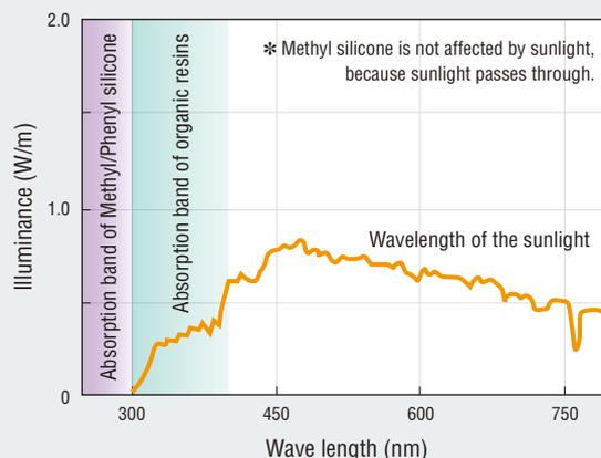
Much of the sunlight reaching the earth's surface is at wavelengths of 300 nm and higher. Most organic resins are susceptible to damage by light in this area of the spectrum. In contrast, Methyl silicone resins absorb almost no light in the UV spectrum, while Methyl/Phenyl silicone resins absorb only light in the spectrum below 280 nm, which means that sunlight has almost no effect.
