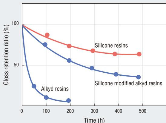
The graph above shows the gloss retention as tested by weatherometer. With an organic resin (alkyd), the drop is dramatic. But the silicone resin and silicone-modified alkyd resin retain much of their original luster.
