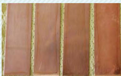
Untreated KBM-403 Epoxy silane Treatment Benzotriazole Treatment X-12-1214A Treatment
