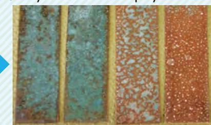
Untreated KBM-403 Epoxy silane Treatment Benzotriazole Treatment X-12-1214A Treatment
