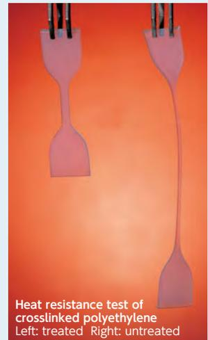
Heat resistance test of crosslinked polyethylene
