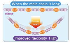
•Model of water repellency and slip property improvement by graft copolymerization of single-end type
