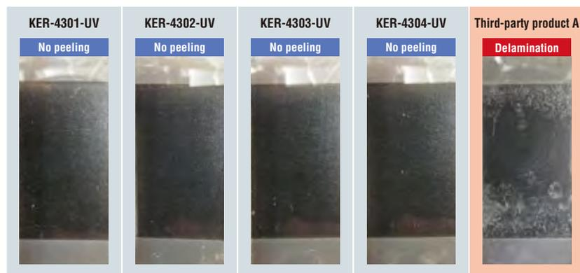
■ Appearance after moisture absorption reflow test
