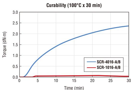
\* Only SCR-4016-A/B is irradiated with UV-light (365 nm UV LEDs: 3,000 mJ/cm<sup>2</sup>)
