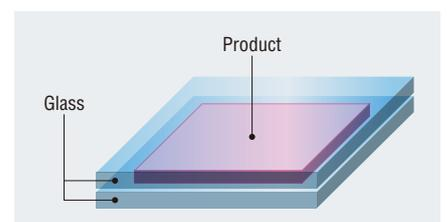
Test method: measured using two glass plates as blanks
