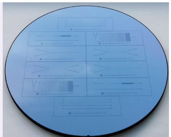
Kyushu Semiconductor KAW Co., Ltd. provides a photo of microfluidic wafers made of UV-PDMS.
